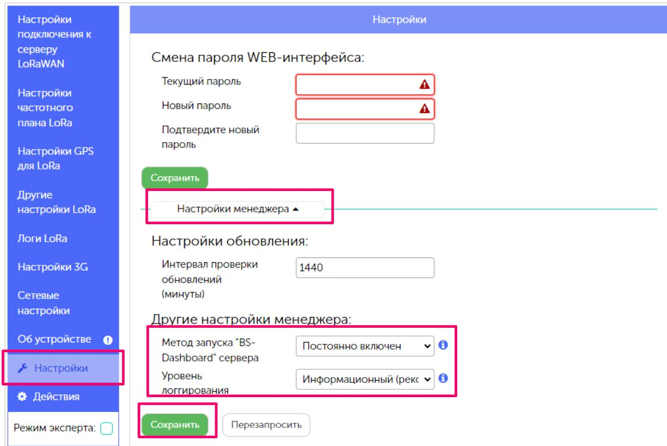
The screenshot shows the configuration interface for the VEGA BS-Dashboard. On the left sidebar, under the 'Настройки' (Settings) menu, the 'Настройки менеджера' (Manager Settings) option is selected and highlighted with a red box. The main panel displays several configuration sections:
